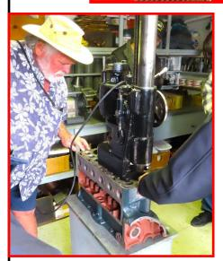
Fred Duerner is examining the cylinder boring machine on a model A engine.
