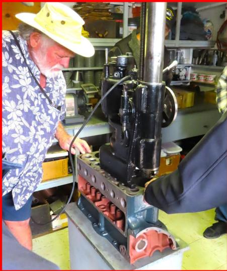
Fred Duerner is examining the cylinder boring machine on a model A engine.
