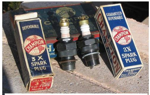
Differences between the NOS and Reproducton Plugs: 3X on the Porcelain of the NOS plug has a rounded top 3; the repro plug has a flat top 3. Knurling on the base of the NOS plug goes all the way to the bottom; repro plug knurling does not. NOS box has red end flaps and does not mention Model B; repro box has blue end flap and mentions A, B. NOS box front says "Dependable"; repro box front says "Guaranteed Dependable". Photo by Rick Black, 20
